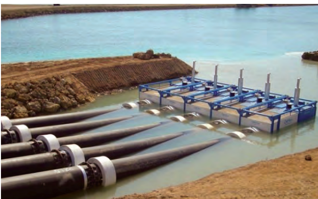
ETEC pumps can handle huge flows of water and are easily assembled in disaster situations. Photos: © ETEC.
