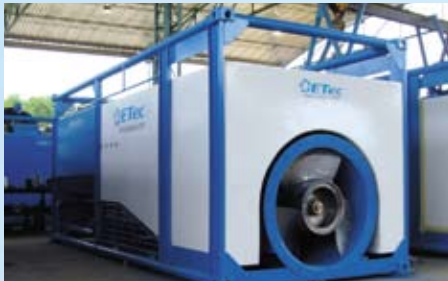
At the heart of the ETEC unit is a PowerTech 6125H engine that drives a high-capacity axial flow pump.
