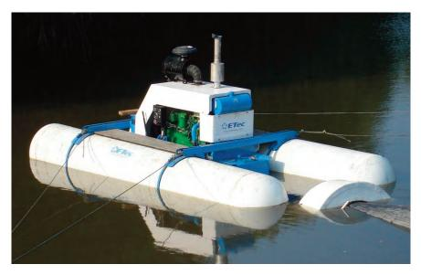
An innovative company in South America designs and builds these high volume floating water pumps. Their pumps are compact, portable, self-contained units that can be quickly and easily set up in a water source. Capable of moving 740 gallons of water per second, these pumps are often used for:
