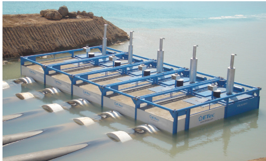
Figure 4. ETEC 48 in floating pumping station.
